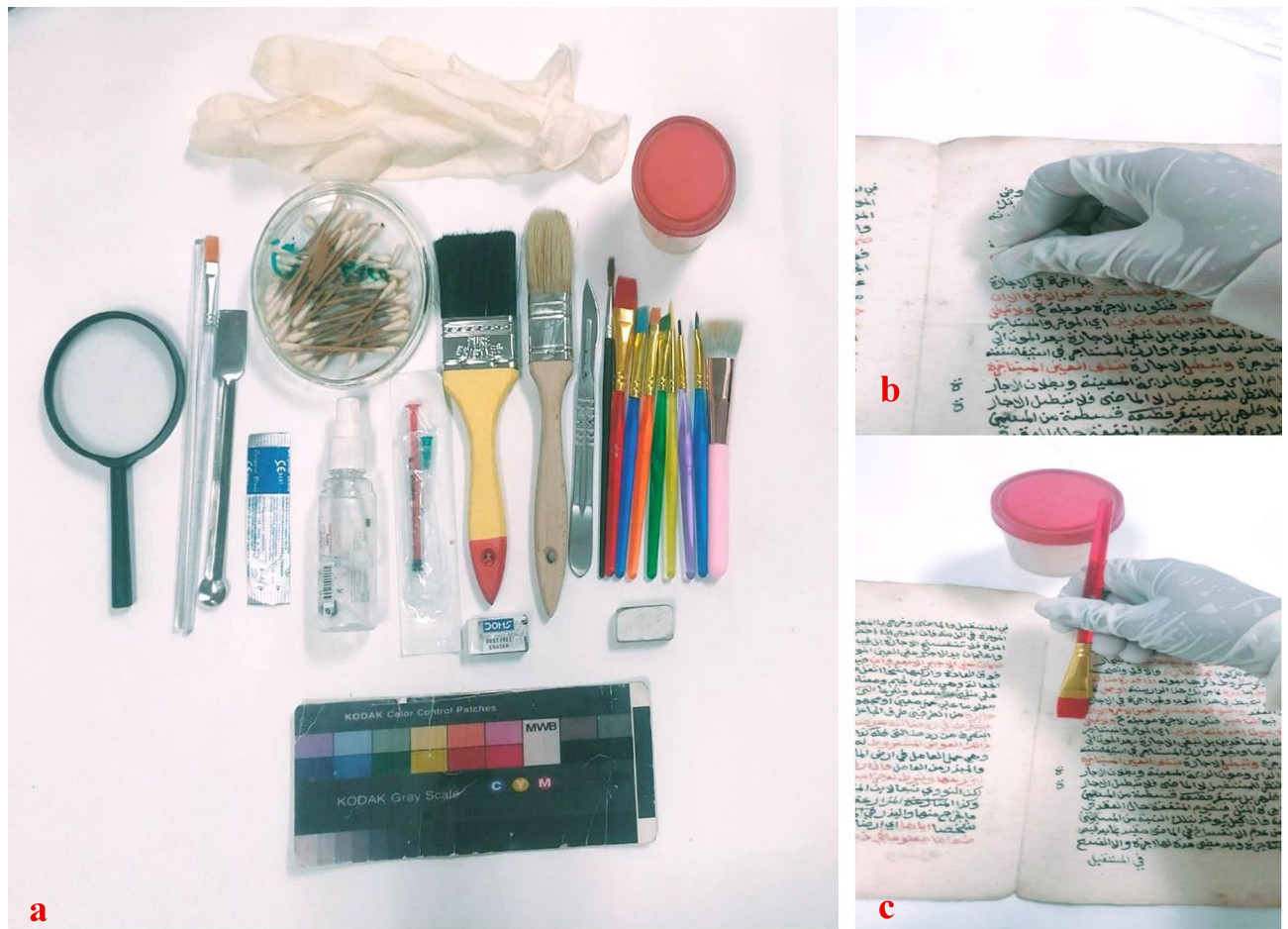
Fig. 18. (a) The tools used in dry cleaning, (b) acid-free erasers, and (c) the application of a consolidation material composed of a 2% concentration loaded with 0.25% of ZnONPs.
