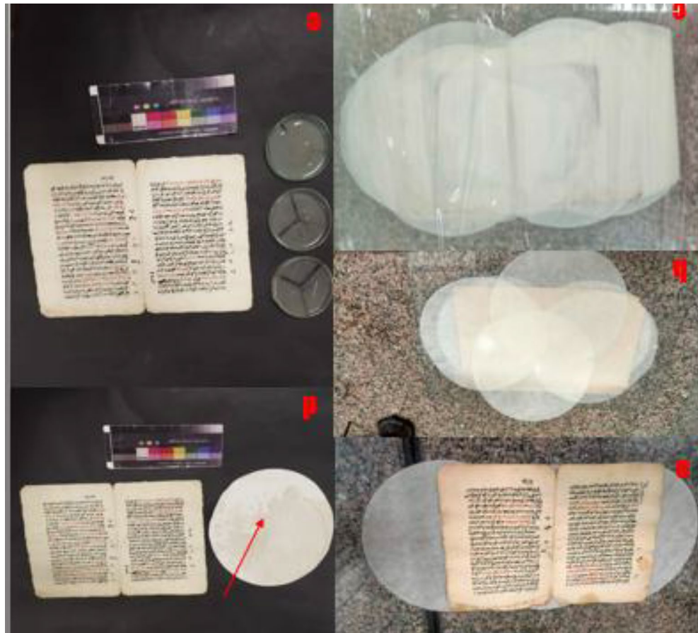
Fig. 17. treatment of the paper manuscript with a geraniol-loaded paper poultice, (a) placement of the manuscript between paper layers, (b) closing the manuscript from all sides, (c) poultice after treatment, showing absorbed dirt and stains, (d) petri dishes confirming inhibition of fungal growth after treatment.
