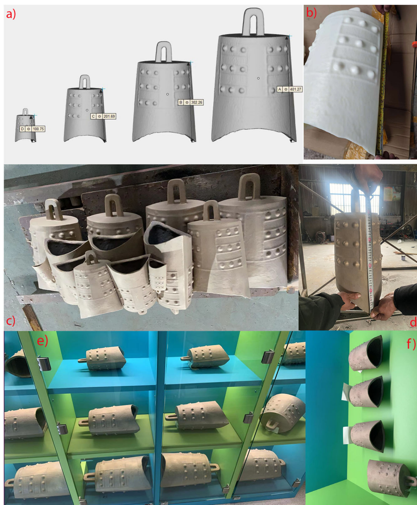
Fig. 4 Brass bells cast by the author's team. a The four different 3D computer models created based on the original Xinzheng Pit16-G2x bell with a side length of 20 cm. The side lengths of the other 3D computer bell models, as specified in the sub-image, are 10 cm (100 mm), 30 cm, and 40 cm respectively. b One of the 3D-printed resin models (Type B, side length 40 cm) based on the corresponding 3D computer model. c Some of the newly cast brass bells. d One of the largest brass bells (Type B, intended side length 40 cm, actual side length 39.6 cm), hung on a frame and ready for testing. e Type A, B, D brass bells stored on a wooden shelf (in total 12). f Type C bells (in total 4). Images and photographs by Chen Xueqing and the author. This figure is not covered by the Creative Commons Attribution 4.0 International License. Reproduced with permission of Kin Sum Li; copyright © Kin Sum Li, all rights reserved.
