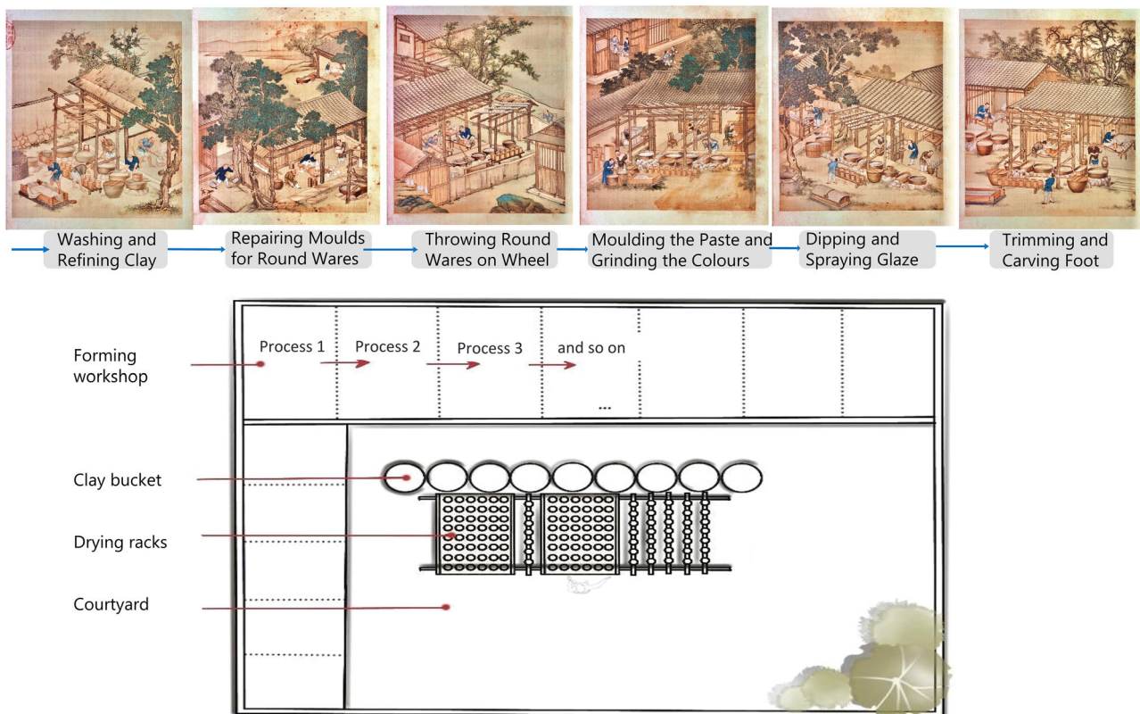
Fig. 19 Aggregation of production processes in courtyard space. Schematic plan showing the aggregation of multiple production processes within a shared courtyard to facilitate logistics and collaboration. Source: This diagram is an original creation by the authors.
