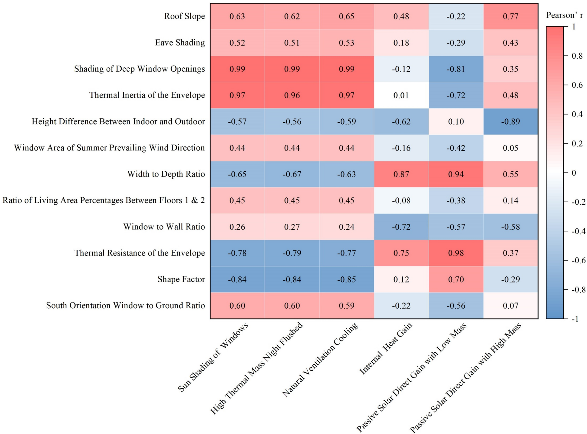
Fig. 5 The correlation analysis results between building factors and passive strategies: the building sample was built between 1600 and 1900
