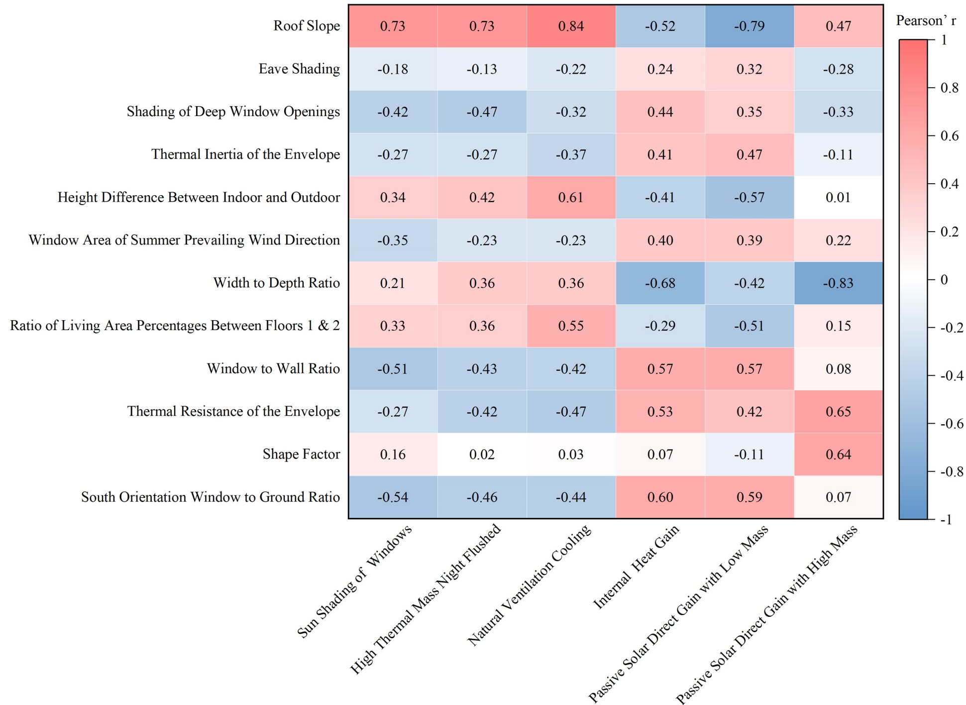
Fig. 6 The correlation analysis results between building factors and passive strategies: the building sample was built between 1900 and 2000
