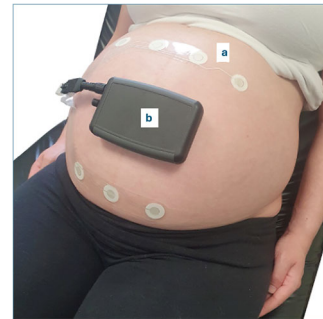
Fig. 1 | Research grade device used in this trial. This figure presents the research-grade device used in the study, consisting of a wearable sensor patch (a) and a hardware unit (b) for acquiring electrophysiological data. The current iteration of the commercial-grade device can be accessed at https://www.kalihealthcare.com/ .
