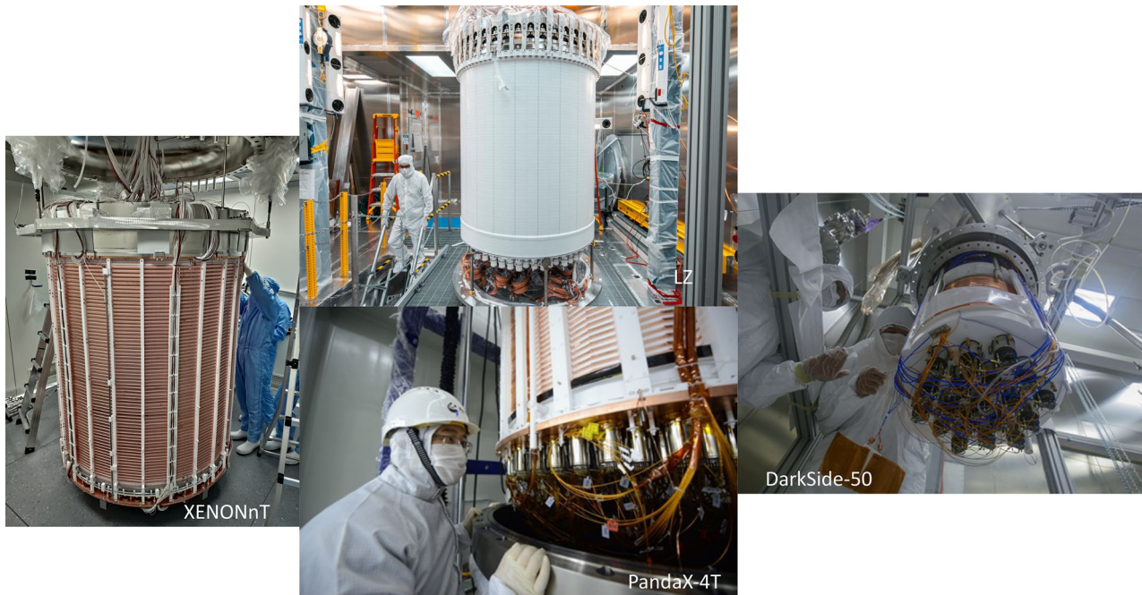
Fig. 3 | Selection of past and currently operating noble liquid TPCs used in the search for dark matter. Shown here are some of the leading experiments employing liquid xenon or liquid argon as a detection target. These detectors operate deep underground to shield them from cosmic rays, and use arrays of photomultiplier tubes (PMTs) to detect scintillation light and ionization signals from particle
