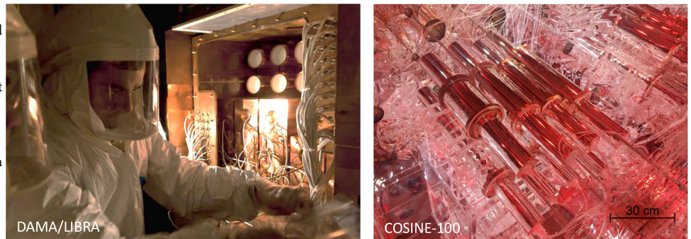
Fig. 9 | Selection of past and currently operating NaI(Tl) detectors. These experiments probe annual modulation signatures expected from Earth’s motion through the dark matter halo. DAMA/LIBRA at LNGS has reported such a signal for about two decades. Independent efforts, including COSINE-100 at the Yangyang Underground Laboratory and ANAIS-112 (not shown in the figure) at the Canfranc Underground Laboratory, aim to test DAMA/LIBRA’s claim. Image credits: ©DAMA/LIBRA Collaboration 176 ; Changhyon Ha for the COSINE-100 Collaboration 177 .
