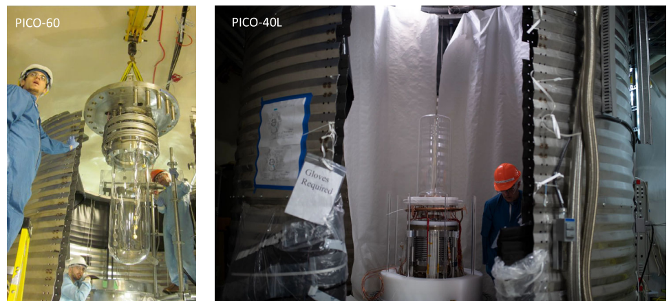
Fig. 8 | Bubble chambers used in the PICO experiment. When a nuclear recoil from a potential dark matter particle interaction occurs in the superheated liquid, it deposits localized energy that triggers the formation of a bubble. Acoustic sensors and cameras record the event, allowing discrimination between NR signals and ER backgrounds. Operated deep underground at SNOLAB, the PICO series of detectors has achieved world-leading sensitivity to spin-dependent WIMP-proton interactions. Shown here are PICO-60 (Credit: Eric Vázquez Jáuregui from the PICO Collaboration 174 ) and PICO-40L (Credit: PICO Collaboration 175 ).
