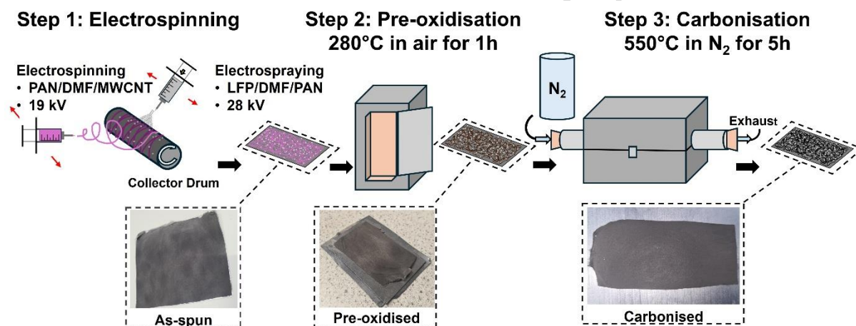
Figure 7. Schematic of the electrode fabrication process with corresponding images of the electrospun mat at each stage. Step 1: Co-electrospinning and electrospaying of PAN/DMF/MWCNT and LFP/DMF/PAN solutions. Step 2: Pre-oxidation at 280 °C for 1 hour (1 °C/min ramp-up, 5 °C/min ramp-down). Step 3: Carbonization at 550 °C for 5 hours (1 °C/min ramp-up, 5 °C/min ramp-down)
