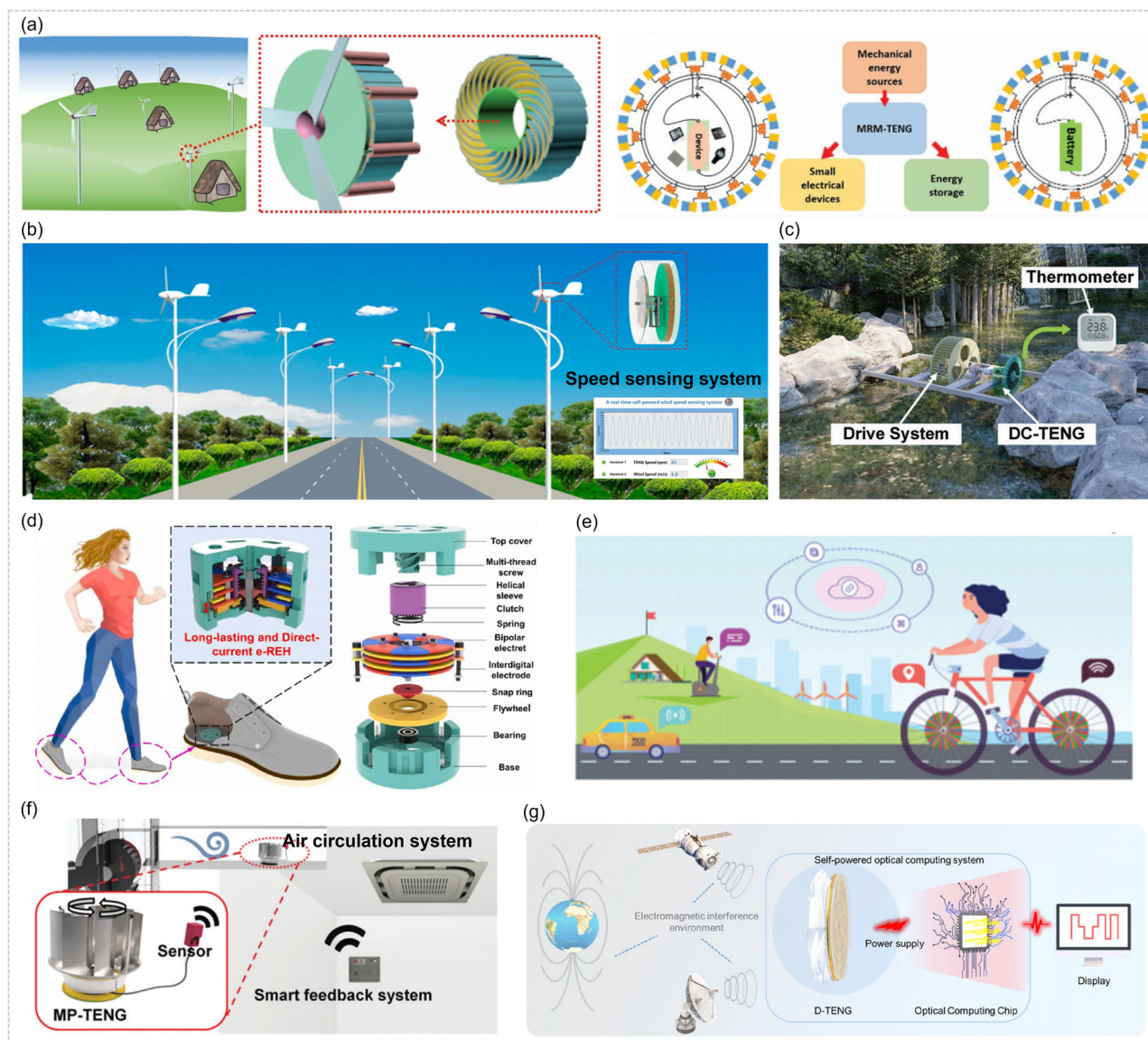
Fig. 9 | The application of the CV-TENG. a Harvesting the wind energy to direct power to small electronics or store the energy in a battery. Reproduced with permission from ref. 43, copyright (John Wiley and Sons, 2020). b Self-powered wind sensor by charge excitation phase-shift TENGs. Reproduced with permission from ref. 56, copyright (Springer Nature, 2023). c Water flow energy harvesting to power sensors. Reproduced with permission from ref. 53, copyright (John Wiley and Sons, 2023). d The CV-TENG was placed in the bottom of human shoes and used to collect human walking, running, and other sports energy. Reproduced with permission
