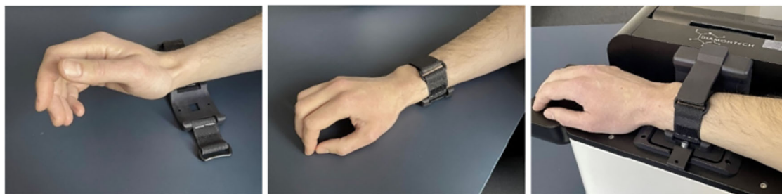
Fig. 4 | Photographs showing the use of a wristband to ensure reproducible attachment to the D-Base. Left: open wristband; center: closed wristband; right: wristband attached to D-Base.
