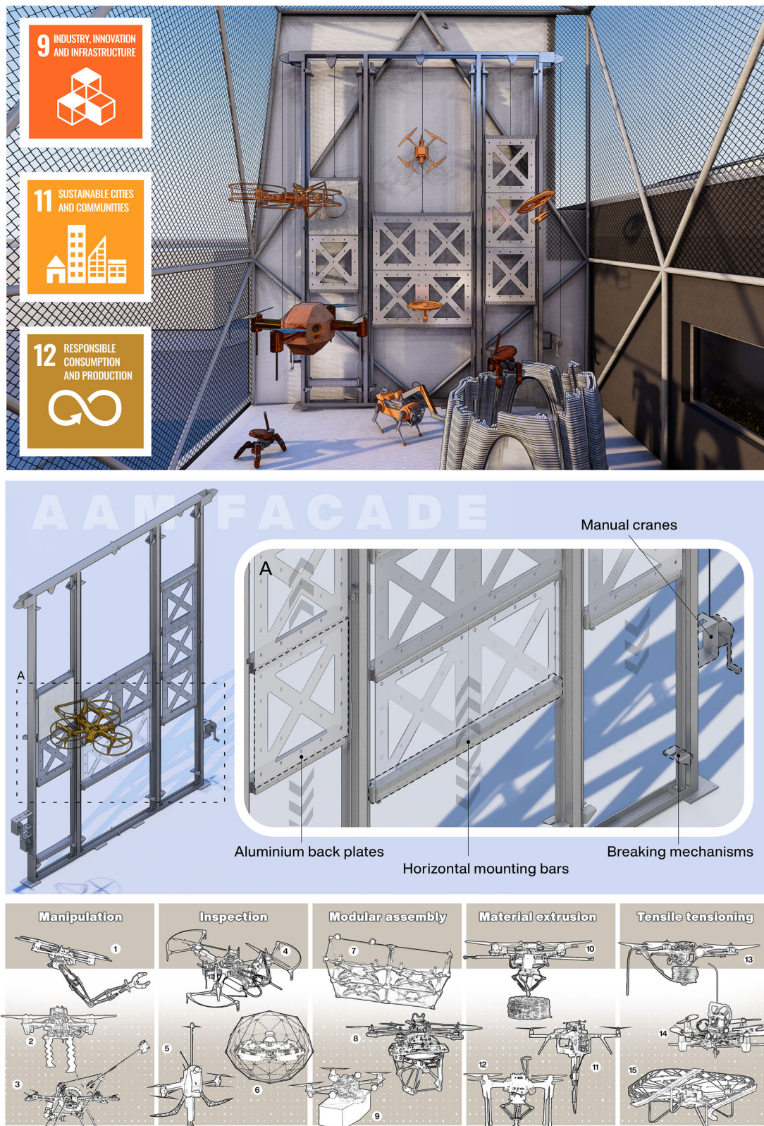
Fig. 5 | (Top) The “Construction Robotics Zone” includes the “Aerial AM Wall” with several example robots and structures and the SDGs targeted. (Center) The “Aerial AM Wall” lift mechanism hosts three liftable columns with different widths. The modular structure of the mechanism consists of aluminium back plates and horizontal mounting bars that can be deployed as needed. (Bottom) Instances of main features of robotic research to be further developed in the “Construction Robotics Zone” and example landmark robots for each feature. (1) Protocentric
