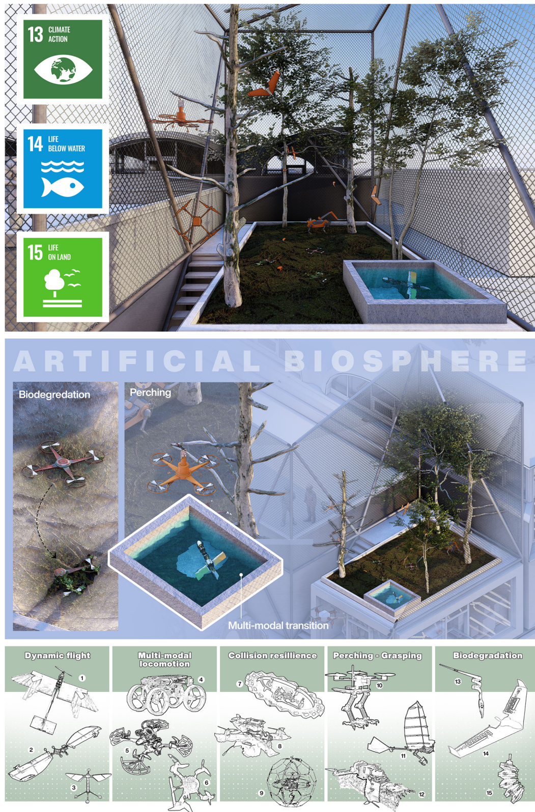
Fig. 4 | (Top) The “Robotics Biosphere Zone” consists of modular artificial trees and soil pots for biodegradation experiments. (Center) A close-up look at the example use cases of the biosphere. (Bottom) Several examples of the robotic testbed are depicted for each capability instance for environmental sensing. (1) Bio-inspired morphing wing drone 65 , (2) Revolving-wing drone 92 , (3). Flapping-wing microscale drone 93 , (4) Multi-modal mobility morphobot (M4) 66 , (5) Hitchhiker multi-modal
