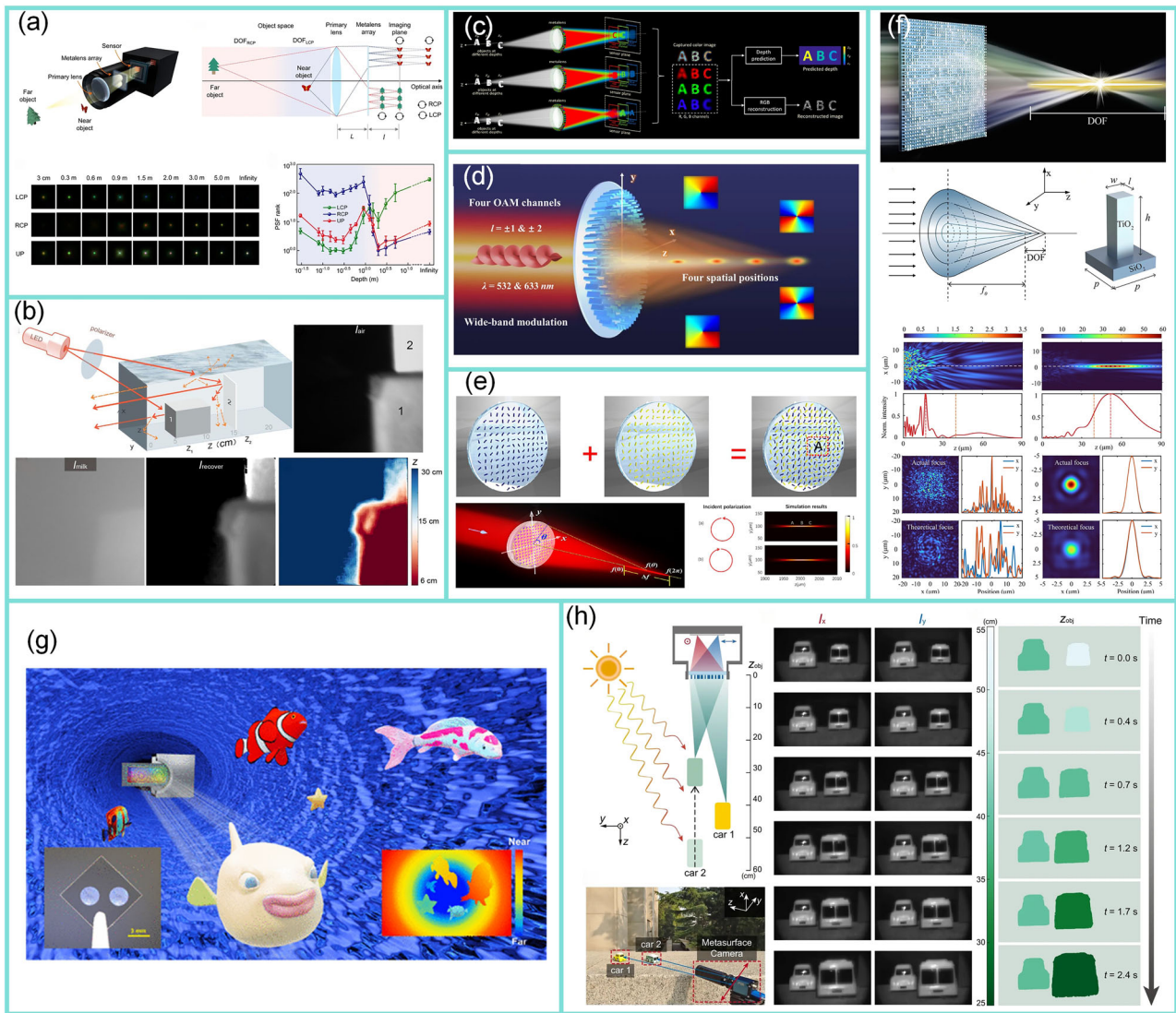
Fig. 4 | Metasurface in extending the depth of field in imaging systems. a Trilobite-inspired neural nanophotonic light-field camera with extreme depth-of-field 74 . b Metalens-assisted system for underwater imaging 75 . c 3D imaging using extreme dispersion in optical metasurfaces 76 . d Active multiband varifocal metalenses based on orbital angular momentum division multiplexing, covering focal
