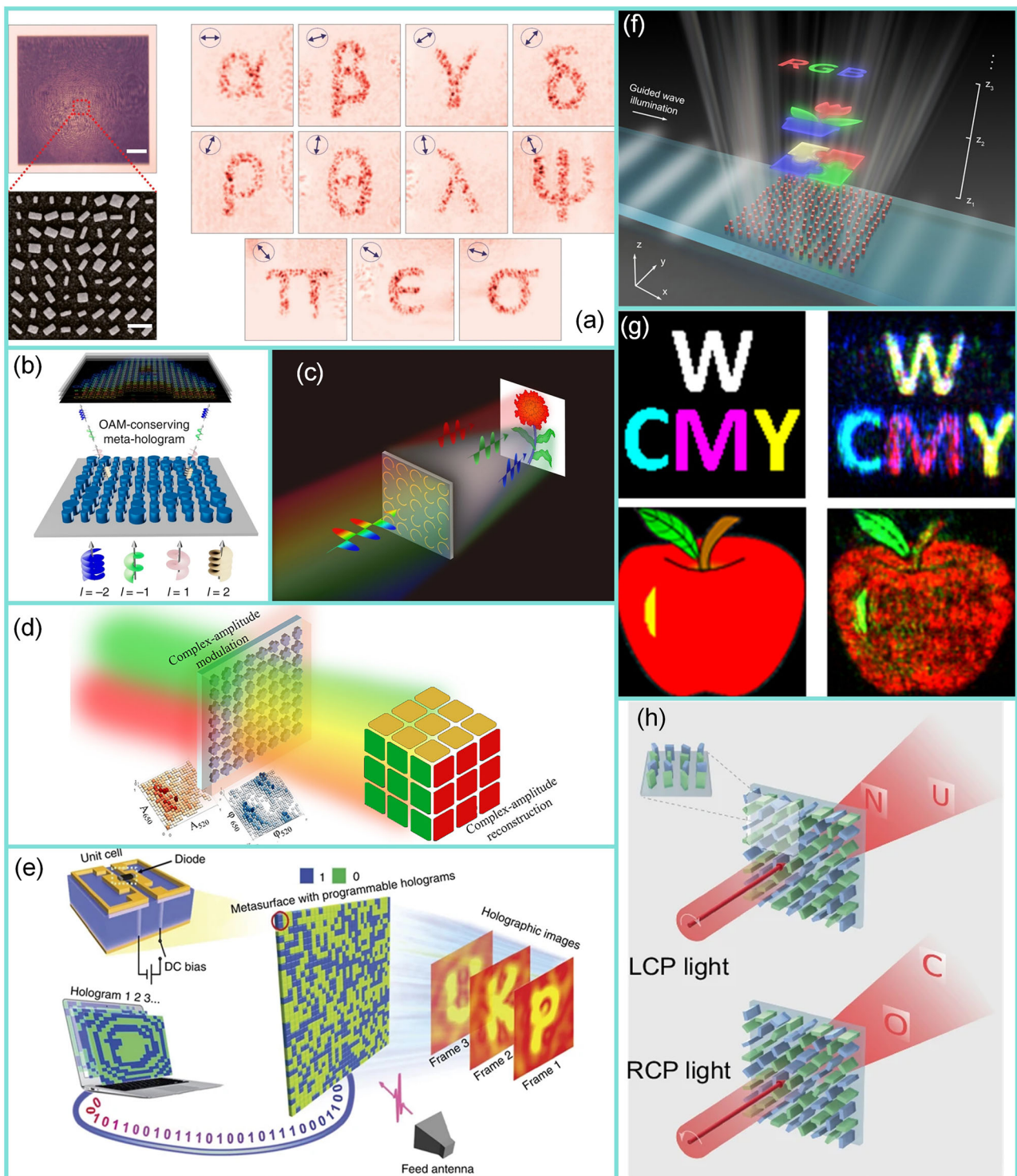
Fig. 8 | Holographic field reconstruction using metasurfaces. a Metasurface-based holographic reconstruction using polarization multiplexing 7 . b Metasurface orbital angular momentum holography 186 . c Wavelength de-multiplexing metasurface hologram 187 . d Color holographic display based on complex-amplitude metasurface 191 .
