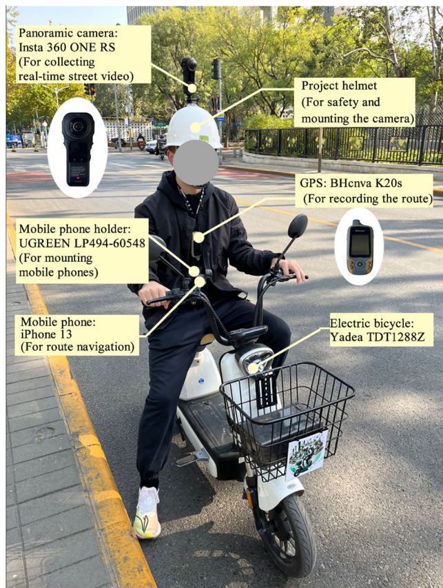
Fig. 3 | Data collection devices. This figure illustrates the equipment and configuration of the Rotating Mobile Monitoring (RMM) method. A researcher is shown on an electric bicycle outfitted with the necessary data collection devices. Key components, identified with labels, include the helmet-mounted 'Insta360 ONE RS' panoramic camera for collecting 360-degree street view video, a handheld GPS unit for recording the precise route, and a smartphone mounted on the handlebars for route navigation. The project helmet serves both for safety and as a stable platform for the camera.
