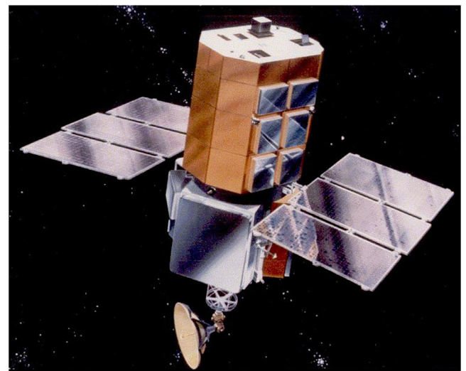
Fig. 1 | Image of the Solar Maximum Mission satellite, first repaired on orbit in 1984 by astronauts James van Hoften and George Nelson during a Space Shuttle servicing mission. The operation restored SMM’s instruments and demonstrated complex rendezvous and hands-on servicing techniques that established confidence and methods later adopted by robotic and commercial on-orbit servicing efforts. Credit: NASA Marshall Space Flight Center (NASA-MSFC).
